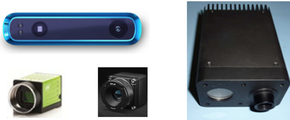
Figure 2. 3D Scanner, Visible Camera, Thermal Camera and LIDAR Candidate Sensors for CCIA System (Shown approximately at approximately two-thirds of real size)
